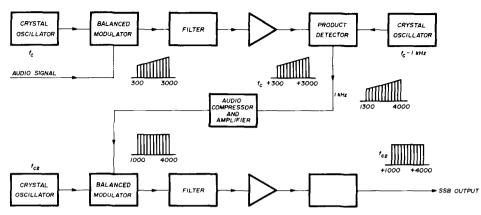
fig. 2. Block diagram of PAØKT's method of achieving an ssb signal with constant amplitude using a fast-acting audio compressor with an offset technique that produces a residual carrier at 1 kHz so that full output can be obtained during pauses in speech.
